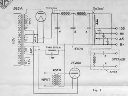
rectifier and power amplifier tubes. There is also another low voltage secondary of 2.5 volts which is primarily intended for use in conjunction with the 226 or 227 types of tubes when this unit is used in a complete two or three stage amplifier.
